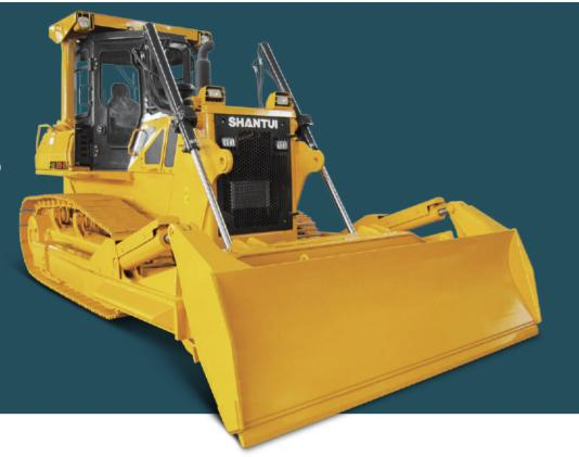
STR20-5 Trimming Dozers feature the high technological content, reasonable design, high power and high productivity, widely used for unloading and cleaning of the bulky materials in cabin, port, power plant and others. In all, the STR16 Trimming Dozers are essential to large wharf.
