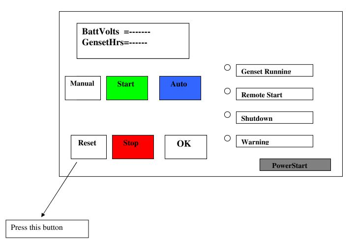
Once you press this push buttons all LED's will glow for 1 second. And LED above STOP button will start bblinking continuosly. While as on display show message shown as in above picture.
