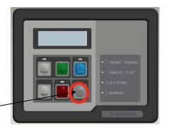
Press **Ok** button to stop the scrolling and enter scroll stop to monitor the parameters on specific screen continuously. How to exit from the Scroll Stop Monitor mode?
