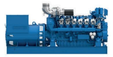
Number of cylinders Bore and stroke Total displacement Engine rotation Idle speed 12V @ 90° 150 x 185 mm 39.2 L Counterclockwise 650 rpm
