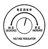
This regulator is used to control the output voltage. Turn the regulator to clockwise to increase the voltage and counter clockwise to decrease it.
